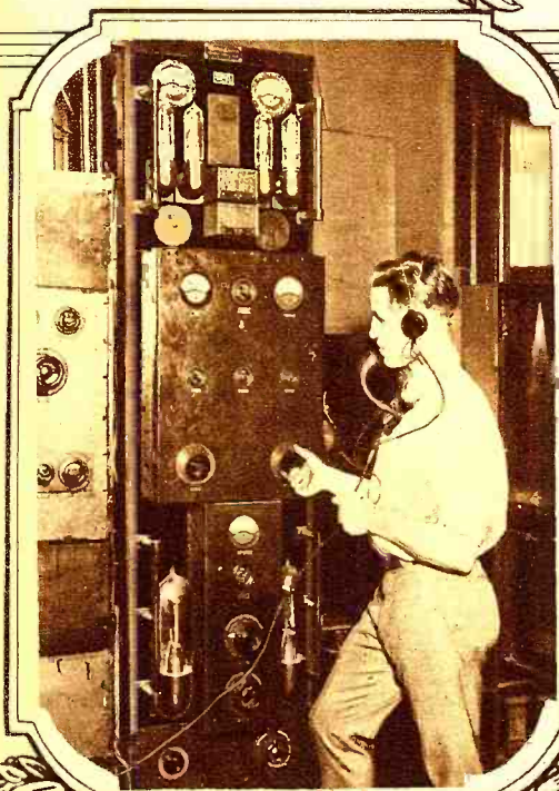
The Four-Stage Vacuum Tube Amplifier in the Laboratories of the Western Electric Company. Passengers on Liners Going Down the Hudson Can Plainly Hear Farewell Messages. © Fotograms.
