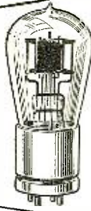
Vacuum tube doing triple duty as amplifier of reflexed audio as well as received and reflexed radio frequency currents, with Erla synchronizing radio and audio transformers
